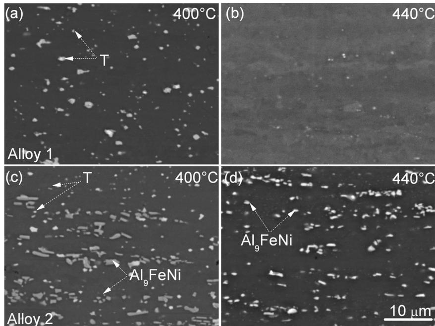
Fig. 1. SEM microstructures of alloy 1 (a, b) and alloy 2 (c, d) after 20 min of annealing at 400 °C (a, c) and 440 °C (b,d).
