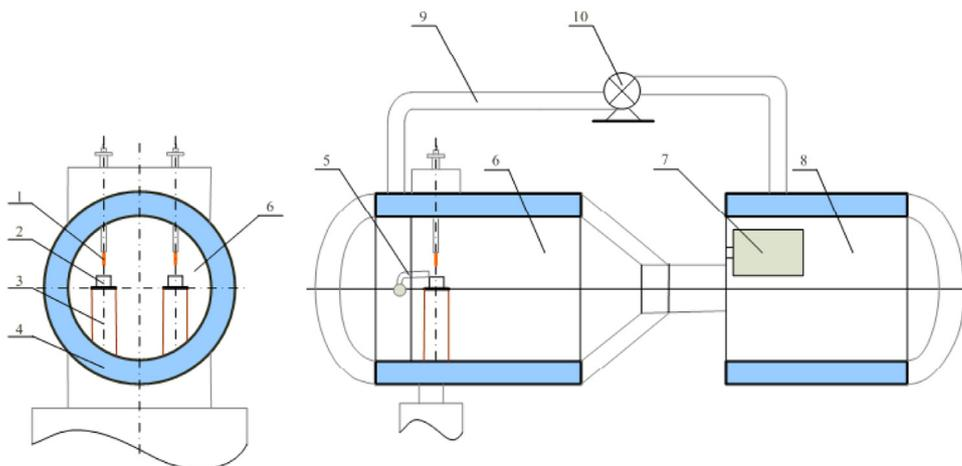
Fig. 1. Schematic drawing of device of continuous preparing nanometer-scale metallic powders (1 Tungsten electrode; 2 Crucible; 3 Water-cooled copper mold; 4 Water-cooled chamber; 5 Pressure gage; 6 Work chamber; 7 Filtration fabric; 8 Collected chamber; 9 Circulating gas path; 10 Circulating fan).
