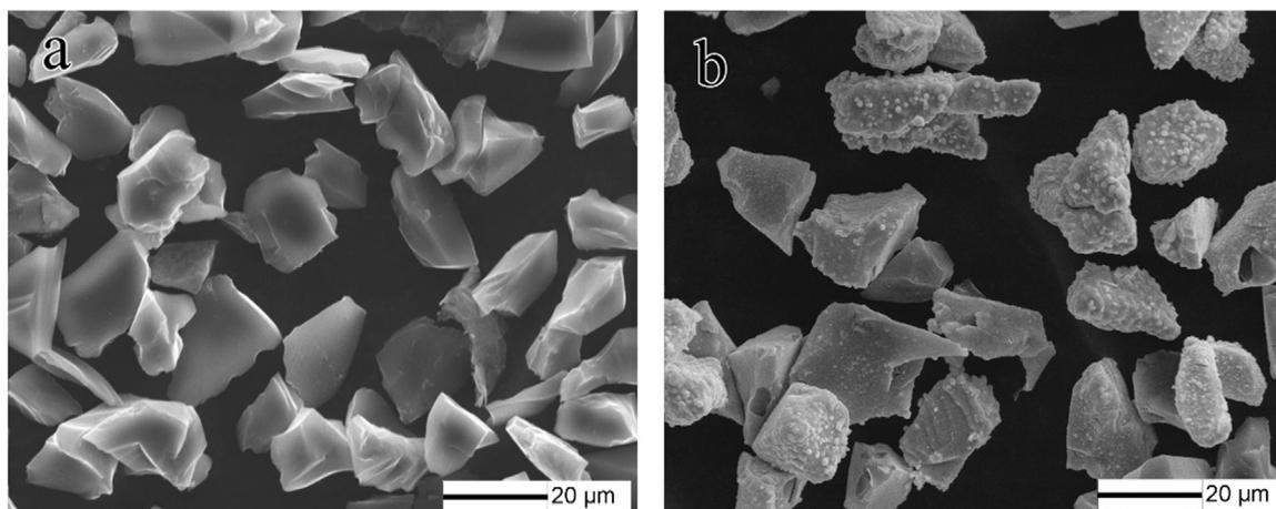
Fig. 1. SEM images showing the morphology of (a) initial  $\text{B}_4\text{C}_p$  and (b) as-coated  $\text{B}_4\text{C}_p$ .
