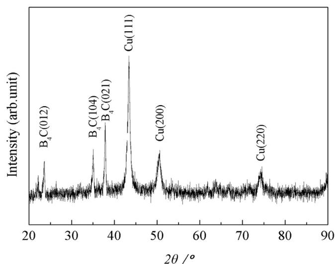
Fig. 2. XRD pattern of the as-coated  $\text{B}_4\text{C}_p$ .
