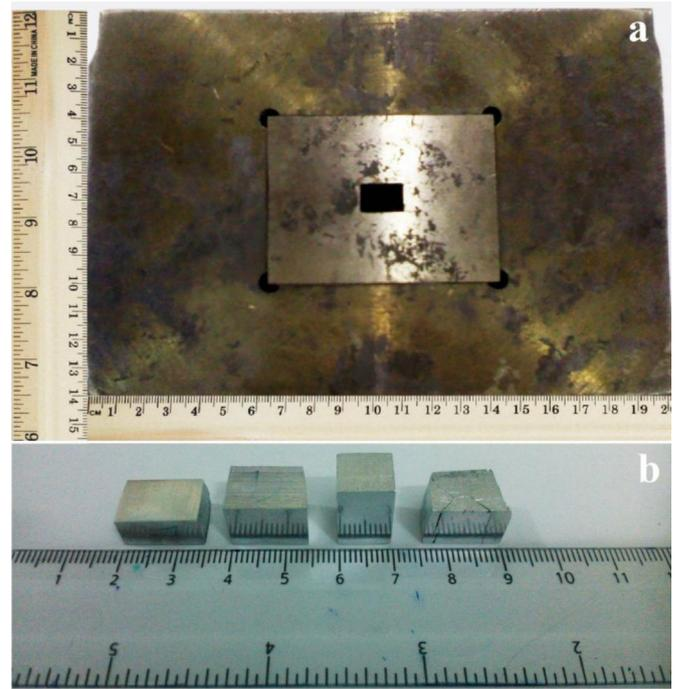
Fig. 2. Illustrations of (a) utilized MDF die, and (b) one-to-four pass MDFed AA5056-H38 alloy specimens.
