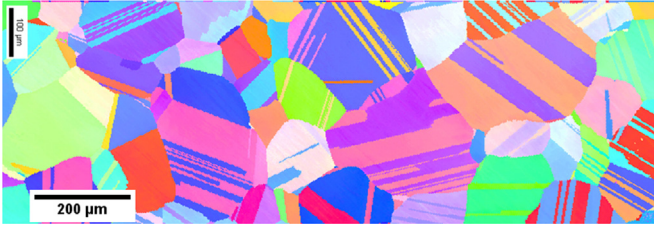
Fig. 1. Inverse pole figure (IPF) map of L-605 after the heating step and before compression.
