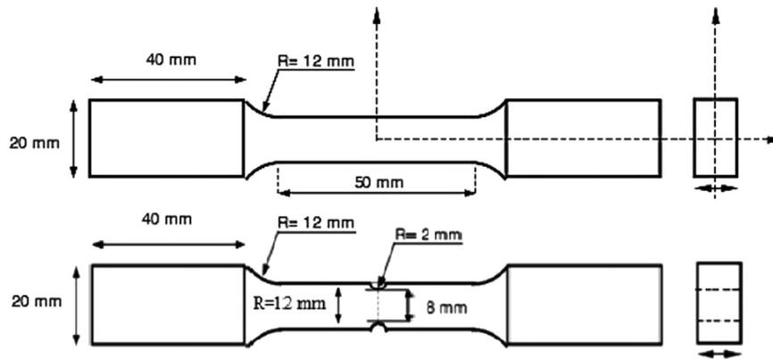
Fig. 1. Schematic representation of tensile specimens, un-notched specimen was named as R and notched specimen named as R2.
