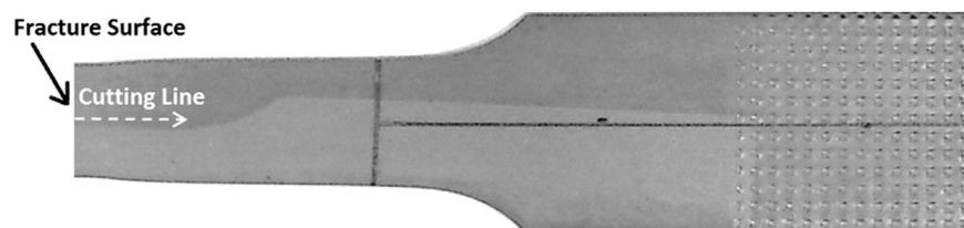
Fig. 2. Specimens was sectioned along the line shown in this image.
