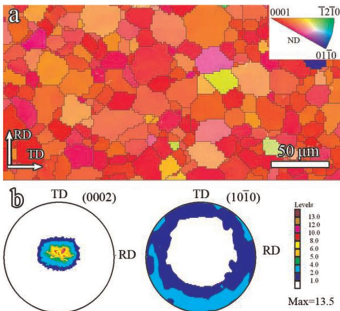
Fig. 1. (a) Inverse pole figure maps and (b) pole figures (acquired by XRD) of the hot-rolled Mg AZ31 plate used in the present study.
