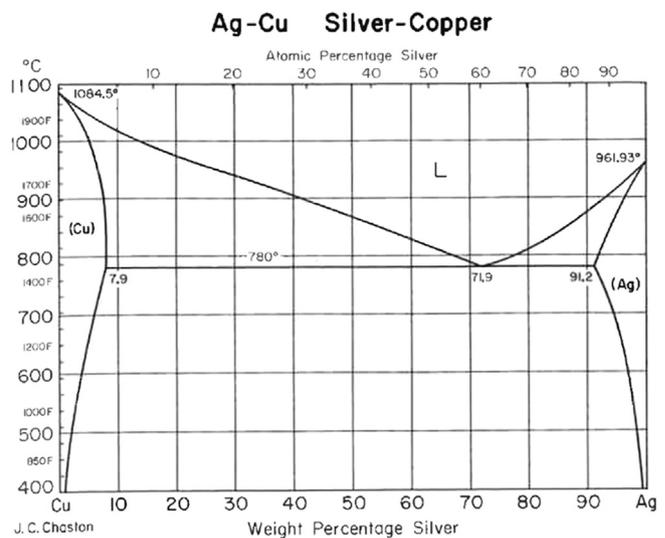
Fig. 1. : Silver–copper phase diagram [1].
