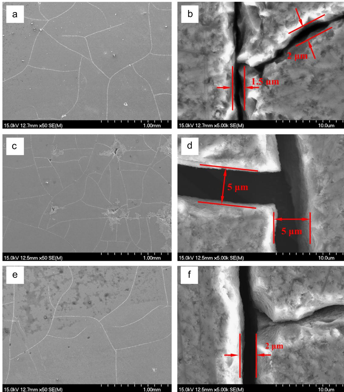
Fig. 1. SEM micrographs for specimen surfaces before oxidation: (a) and (b) S1; (c) and (d) S2; (e) and (f) S3.
