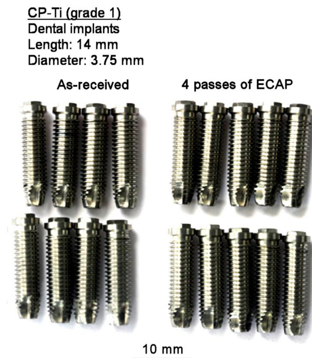
Fig. 1. Dental implants used in the experiments. Left: implants machined from the as-received material. Right: implants machined from the material processed by ECAP.
