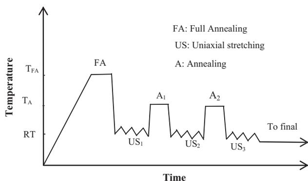
Fig. 1. A schematic illustration of MUSA process.
