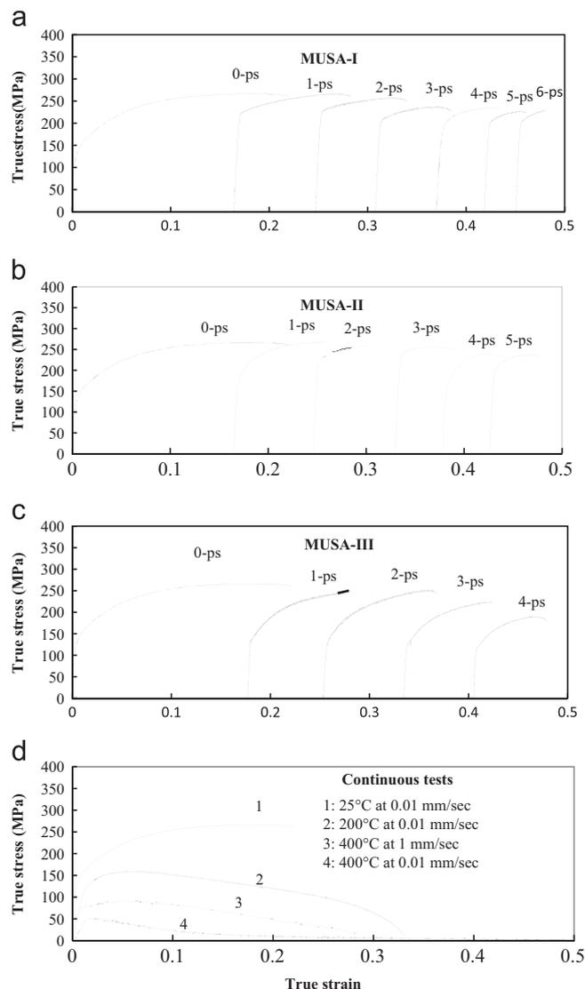
Fig. 2. Stress–strain curves of AZ31 deformed by (a) MUSA-I, (b) MUSA-II, (c) MUSA-III and (d) continuous tests to fracture.
