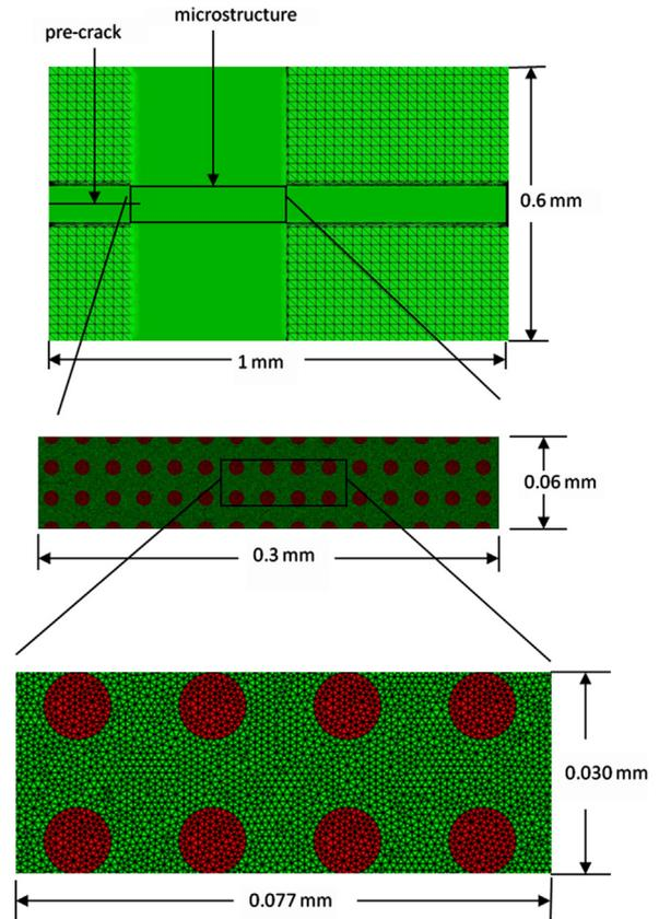
Fig. 1. Finite element discretization and a sampled microstructure of bimodal NS Cu. (For interpretation of the references to colour in this figure, the reader is referred to the web version of this article.)
