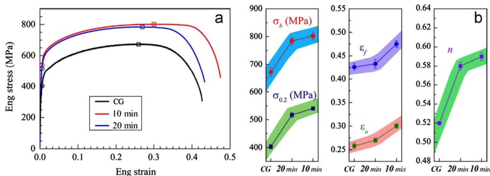
Fig. 1. (a) Tensile engineering stress vs. strain curves; (b) simultaneous increase of mechanical properties such as yield stress ( $\sigma_{0.2}$ ), ultimate tensile strength ( $\sigma_b$ ), uniform elongation ( $\epsilon_u$ ), elongation to failure ( $\epsilon_f$ ) and strain hardening exponent ( $n$ ).
