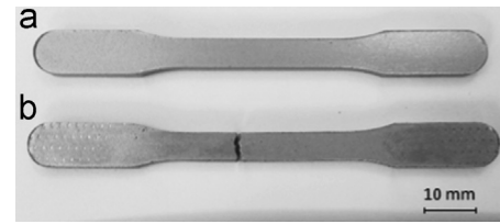
Fig. 1. General view of tensile test specimen sintered at 1150 °C for 1 h; (a) before fracture and (b) after fracture.
