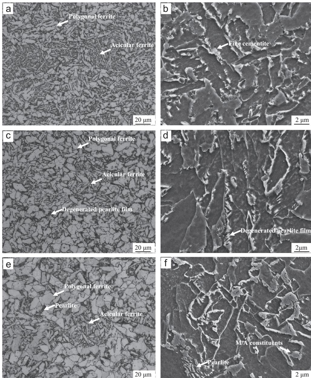
**Fig. 1.** Optical and SEM micrographs of experimental steel at different thicknesses: (a) OM of 1/8; (b) SEM of 1/8; (c) OM of 1/4; (d) SEM of 1/4; (e) OM of 1/2; and (f) SEM of 1/2.
