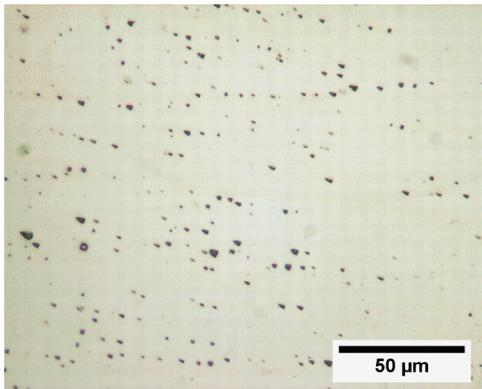
Fig. 1. Etched pits on the surface of the annealed Cr sample gives an averaged dislocation density of about  $1 \times 10^{10} \text{ m}^{-2}$ .
