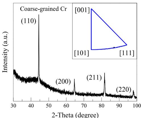
Fig. 2. XRD pattern of coarse-grained Cr and the crystalline orientation of the grain studied.
