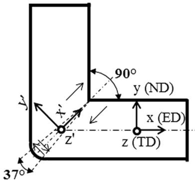
Fig. 1. Die configuration and the reference system used in this study.
