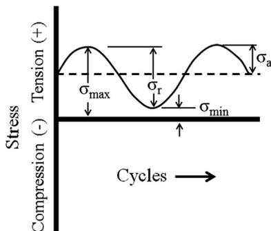
Fig. 2. Repeated stress cycle of the fatigue behavior applied in this study [11].
