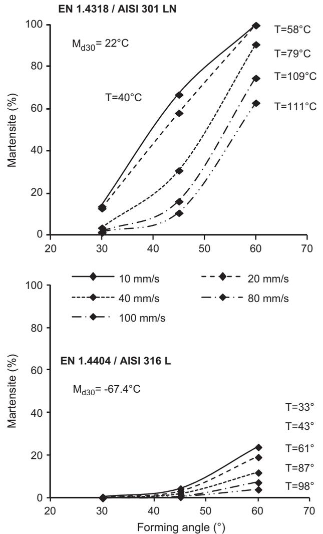
**Fig. 1.** The measured fractions of martensite for AISI 301LN and AISI 316L, as functions of temperature and forming angle.
