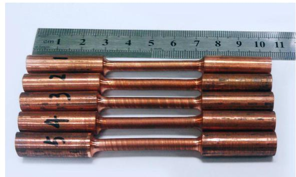
Fig. 2. Photograph of torsional deformed samples.
