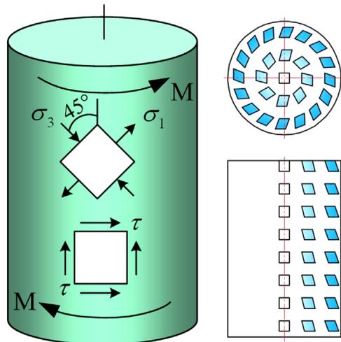
Fig. 1. Schematic diagram of stress and grain-boundary rotation in torsion deformation.
