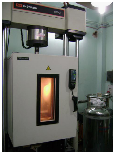
Fig. 1. Experimental set-up for tensile testing at subzero temperatures.
