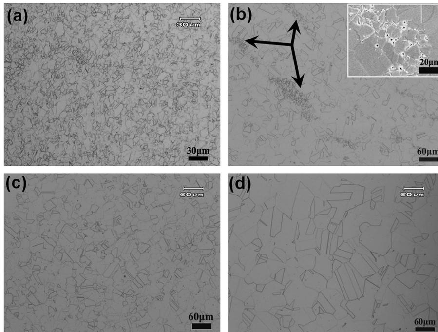
Fig. 1. Optical microstructure of the alloys in (a) as-rolled condition and after solution-treated at (b) 1173 K, (c) 1213 K, and (d) 1253 K. The inset in (b) is the higher magnification image of  $\eta$  phase.
