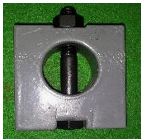
Fig. 1. Jig for applying constant stress state during hydrogen charging.
