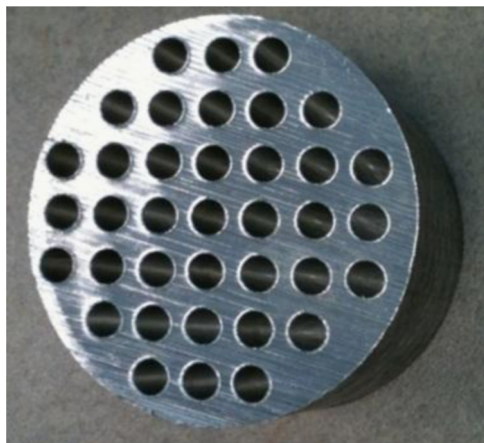
Fig. 1. Array of blind holes in AZ31 disk to be filled by nanoparticles.
