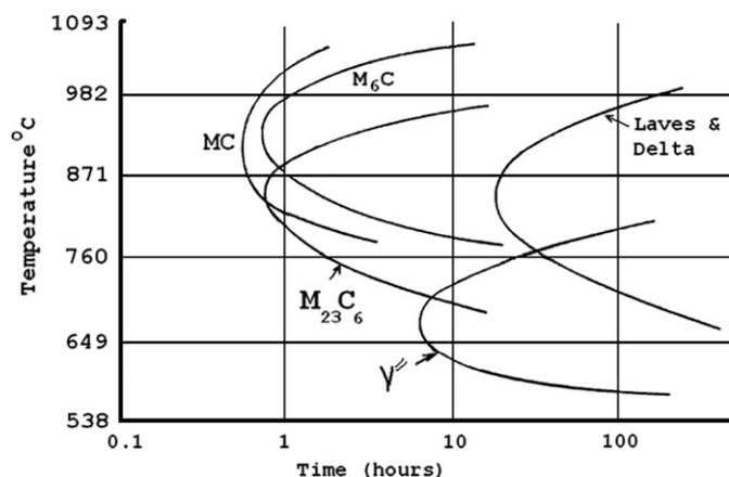
**Fig. 1.** Time–temperature–transformation diagram of Alloy 625 [1].
