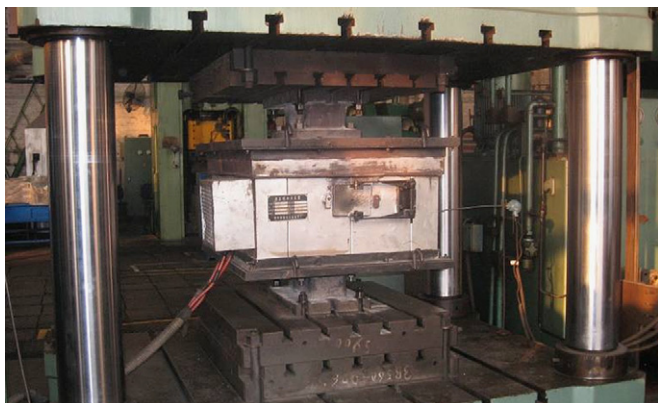
Fig. 1. The hydraulic press and furnace for blades forging.
