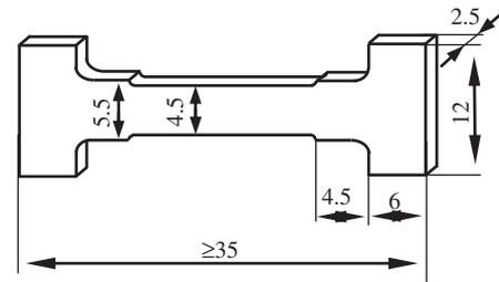
Fig. 1. Schematic diagram of the tensile creep samples.
