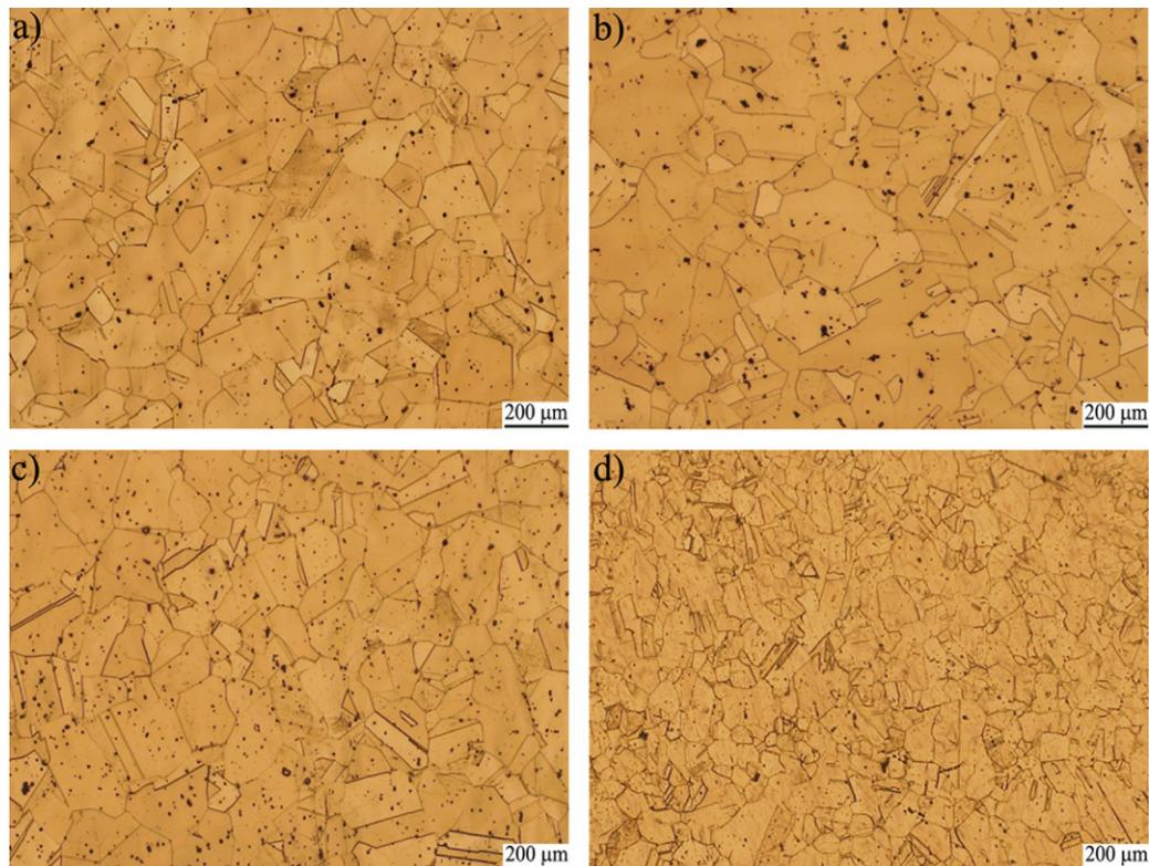
**Fig. 1.** Microstructures of studied TWIP steels after solution heat treatment, previous to hot compression tests: (a) TW-NM steel, (b) TW-Nb steel, (c) TW-V steel and (d) TW-Ti steel.
