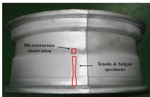
**Fig. 1.** Schematic diagram for specimen preparation in rim section of automotive wheel.
