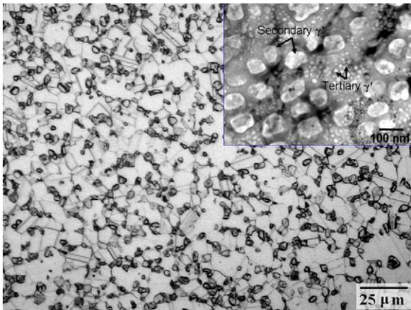
**Fig. 1.** The microstructure of TMW-4M3 alloy. The inset image shows the fine secondary and tertiary  $\gamma'$  precipitates.
