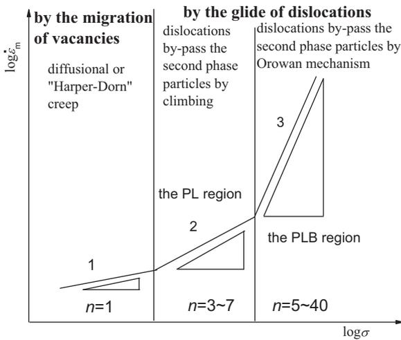
Fig. 1. Minimum creep rate  $\dot{\epsilon}_m$  dependence on applied stress  $\sigma$  for second phase particles strengthened materials.
