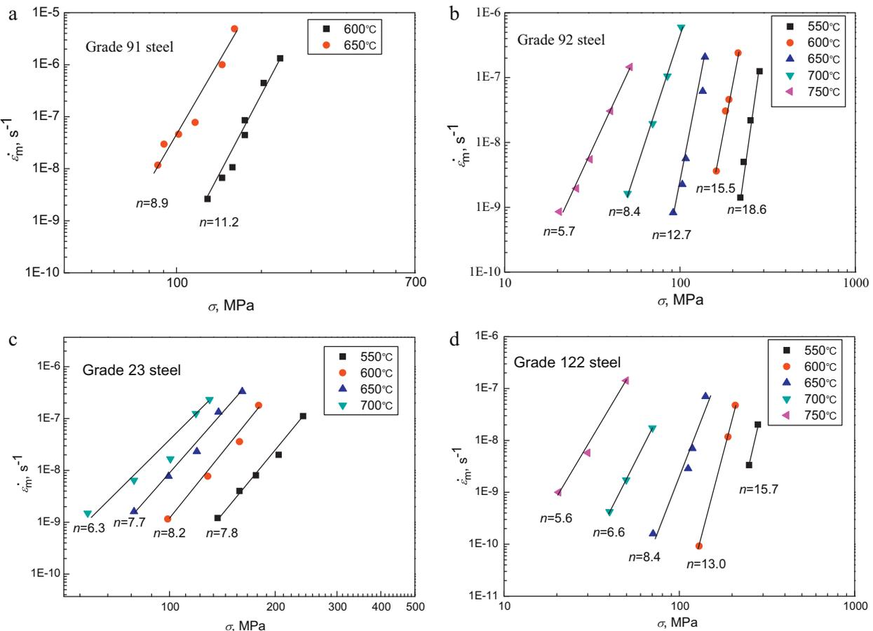
Fig. 2. Minimum strain rate  $\dot{\epsilon}_m$  dependence on applied stress  $\sigma$  at various temperatures for (a) Grade 91 [16], (b) Grade 92 [17], (c) Grade 23 [18] and (d) Grade 122 [19] steels.
