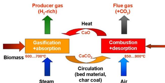
Fig. 2. Steam gasification without selective transport of CO<sub>2</sub>.
