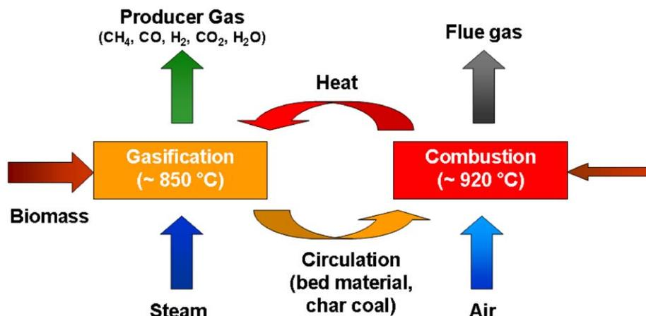
Fig. 1. Steam gasification with selective transport of CO<sub>2</sub>.
