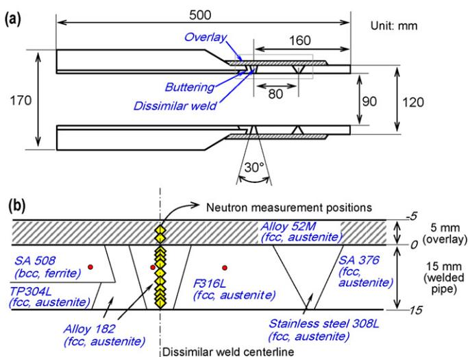
**Fig. 1.** (a) Schematic of the dissimilar weld overlay pipe specimen, (b) measurement locations of the specimen in the neutron-diffraction experiments.
