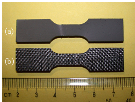
Fig. 1. Geometry of specimens. (a) Coated specimen with a density of 2.05 \text{ g/cm}^3 (b) uncoated specimen with a density of 1.8 \text{ g/cm}^3 .
