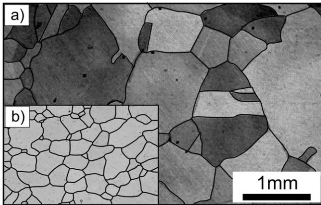
Fig. 1. Initial microstructure of nickel 45% cold worked and annealed at 1180 °C (a) for 48 h with  $D_0 = 770 \mu\text{m}$  and (b) for 1 h with  $D_0 = 240 \mu\text{m}$ .
