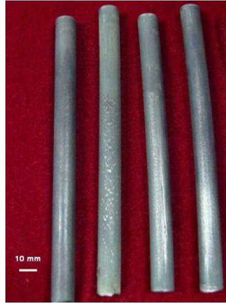
Fig. 2. Photograph of the fine-grained 93W–4.9Ni–2.1Fe–0.03Y alloy bars after rapid hot extrusion.
