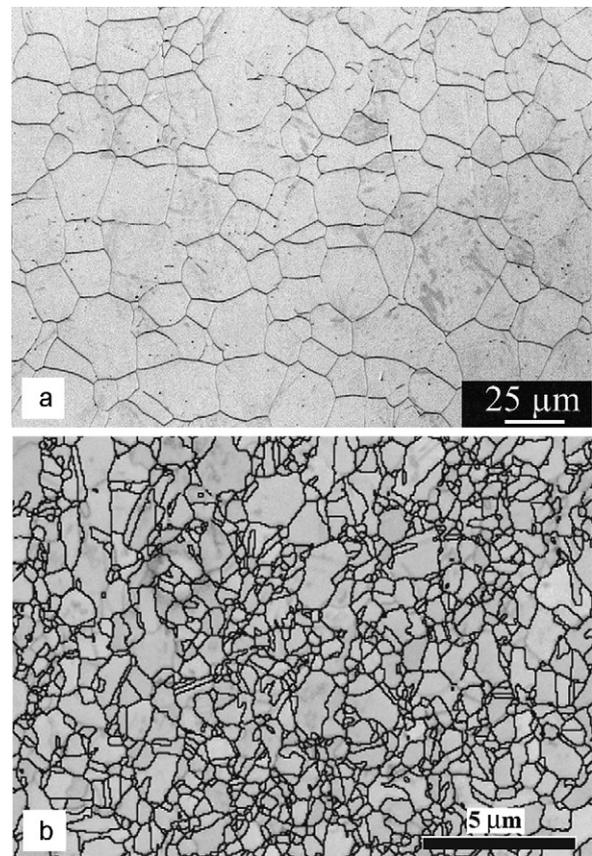
Fig. 1. Grain structure of (a) as-received coarse-grained (CG) sheet (OM) and (b) 50% cold-rolled steel after reversion annealing at 800 °C for 10 s (SEM-EBSD).
