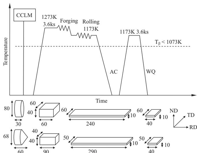
**Fig. 2.** A schematic drawing of the heat treatment for the Ti–5Mo–5Zr alloy with an ingot diameter of 80 mm and for the Ti–10Mo–2Fe alloy with an ingot diameter of 68 mm. CCLM, AC and WQ refer to cold crucible levitation melting, air cooling and water quenching, respectively.
