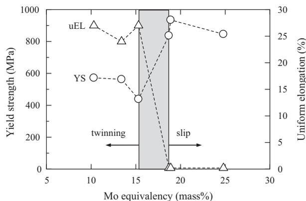
**Fig. 1.** Changes in the yield strength (YS) and the uniform elongation (uEL) with the Mo equivalency in the reference alloys.
