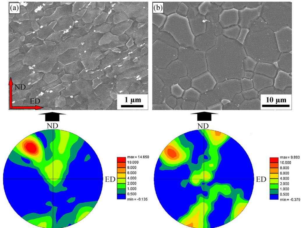
Fig. 1. SEM microstructure and basal plane pole figure of Mg–Zn–Ca alloy processed by (a) ECAP and (b) subsequent annealing.
