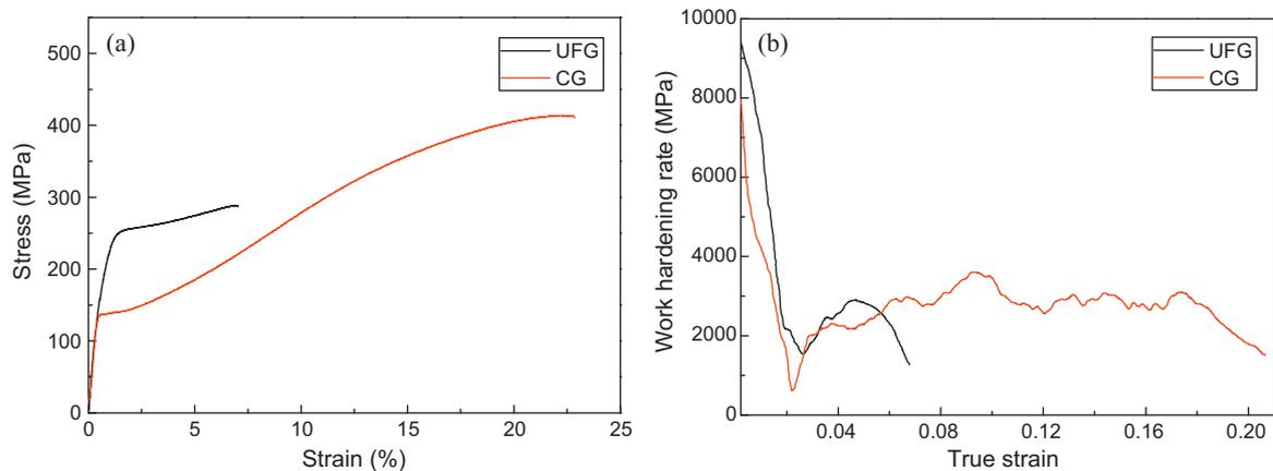
Fig. 2. Mechanical properties of UFG and CG Mg–Zn–Ca alloys: (a) compressive stress vs. strain curves, (b) work hardening rate vs. true strain curves.
