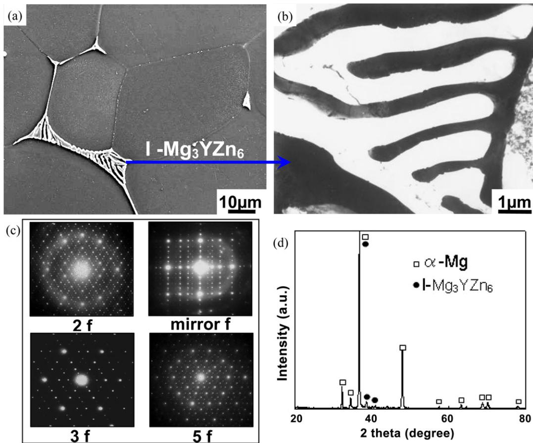
**Fig. 1.** Typical microstructures and XRD pattern of the as-cast ZWK510 alloy specimen. (a) SEM image, (b) TEM micrograph of eutectic I-phase (bright field image), (c) SADP from I-phase exhibiting 2-fold, mirror fold, 3-fold and 5 fold symmetry and (d) XRD pattern.
