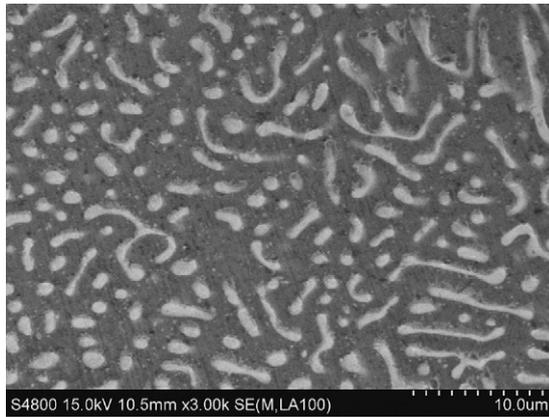
**Fig. 1.** Microstructure of Al–14Cu–7Ce alloy after annealing at 580°C for 3 h obtained from SEM.
