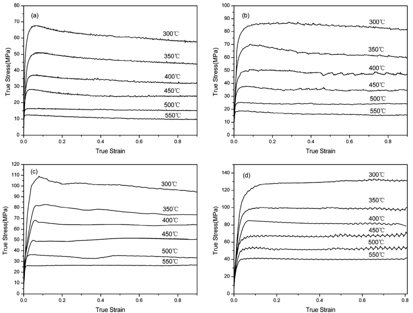
**Fig. 2.** True stress–true strain curves for Al–14Cu–7Ce alloy during hot deformation: (a)  $\dot{\epsilon} = 0.001 \text{ s}^{-1}$ ; (b)  $\dot{\epsilon} = 0.01 \text{ s}^{-1}$ ; (c)  $\dot{\epsilon} = 0.1 \text{ s}^{-1}$ ; (d)  $\dot{\epsilon} = 1 \text{ s}^{-1}$ .
