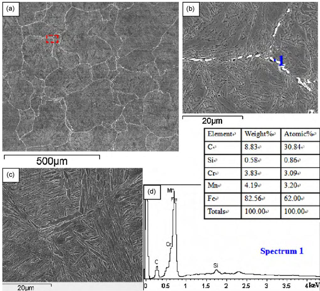
Fig. 2. (a) The SEM morphology of specimen 1. (b) The magnification of the zone within the red dashed line frame in (a). (c) The SEM morphology of specimen 3. (d) The composition analysis on the blue spot in (b). (For interpretation of the references to color in this figure legend, the reader is referred to the web version of this article.)
