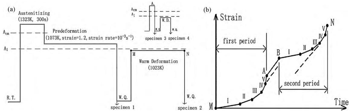
Fig. 1. (a) Schematic diagram of the novel procedure and (b) strain–time curve of the warm deformation step.
