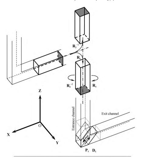
Orientation transformation matrices for the operation of each pressing pass
