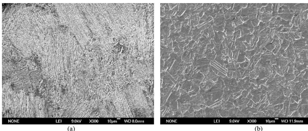
Fig. 2. Microstructures of (a) fully lamellar and (b) duplex TiAl-based alloy.
