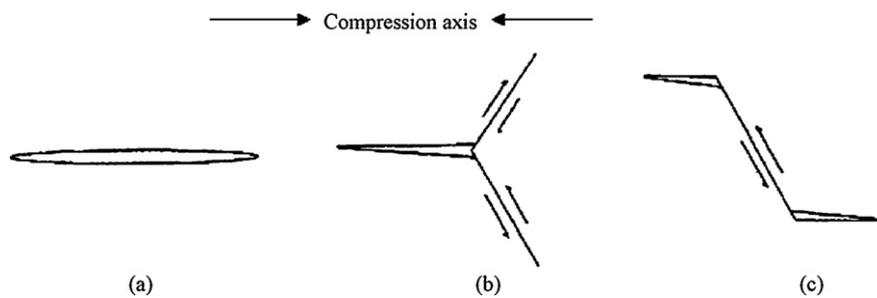
Fig. 1. Three types of crack initiation and propagation in the compression loading mode [9].
