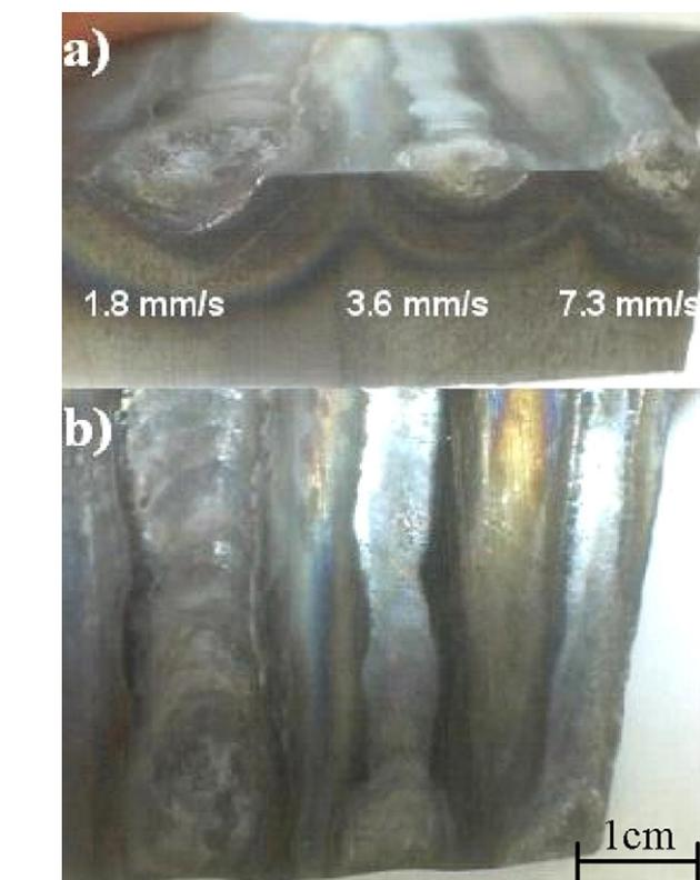
**Fig. 1.** The melted surfaces of GGG 40 using the TIG process at different electrode traveling speeds. (a) Cross-section of the melted surface and (b) top view of the melted surface.
