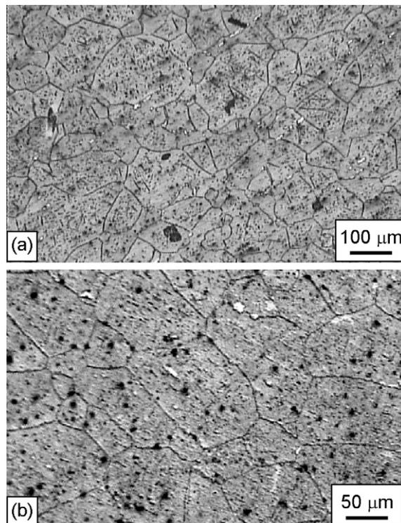
**Fig. 2.** Optical micrographs of the annealed microstructures. (a) LAZ1010 alloy, (b) LAZ1010 alloy on a larger scale.
