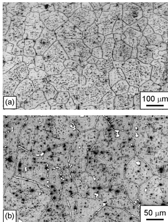
**Fig. 1.** Optical micrographs of the as-extruded microstructures. (a) LAZ1010 alloy, (b) LAZ1010 alloy on a larger scale.
