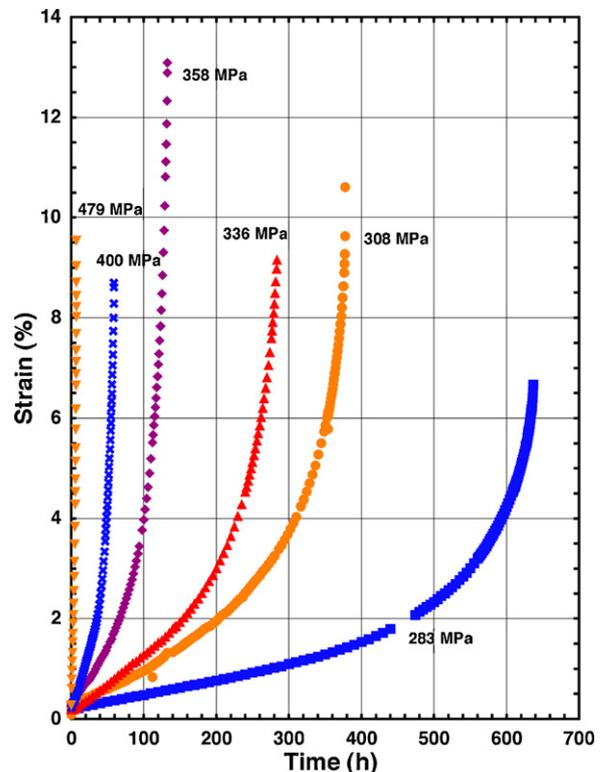
Fig. 2. Creep curves (strain versus time) obtained for different stress levels in air at 850 °C.
