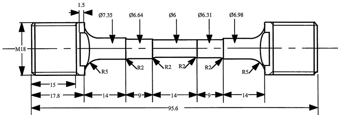
Fig. 1. Geometry of the multiple sections specimen used for creep tests.
