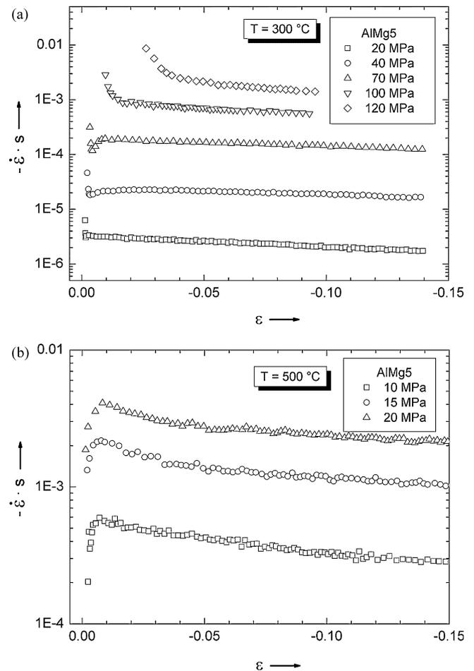
**Fig. 2.** Creep behavior of the non-reinforced AlMg5 matrix alloy at (a) 300 °C and (b) 500 °C.
