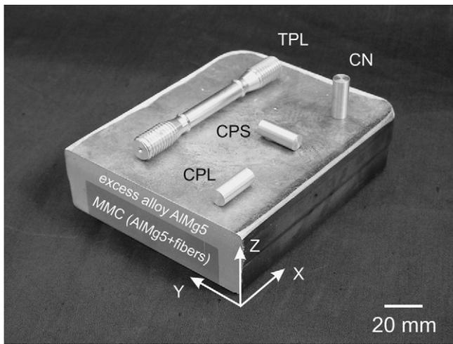
**Fig. 1.** AlMg5-block obtained by squeeze casting. The dark rectangular region in the lower part of the block represents the fiber reinforced MMC (AlMg5 + fibers). The image shows the specimen geometries and orientations considered in the present study.
