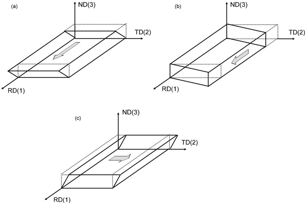
Fig. 2. Schematic diagram showing shear strains developed during rolling. (a)  $\dot{\epsilon}_{13}$ , (b)  $\dot{\epsilon}_{12}$  and (c)  $\dot{\epsilon}_{23}$ .
