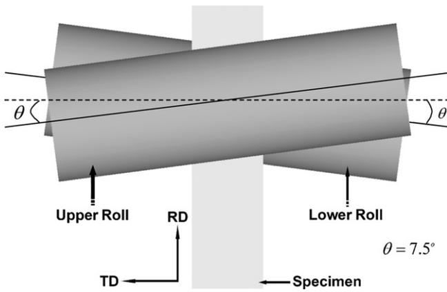
Fig. 1. Schematic diagram of the cross-roll rolling mill (top view).
