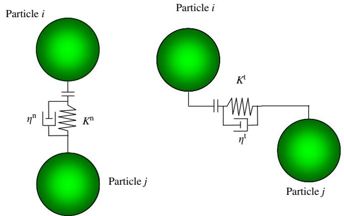
Fig. 1. Schematic drawing of Voigt elements between a pair of particles in normal and tangential directions.
