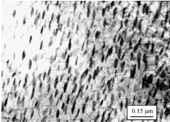
Fig. 1. TEM microstructure of  $Ti_2Cu$  intermetallic particles in the Ti–2.5Cu alloy after solution treatment and two-step aging.
