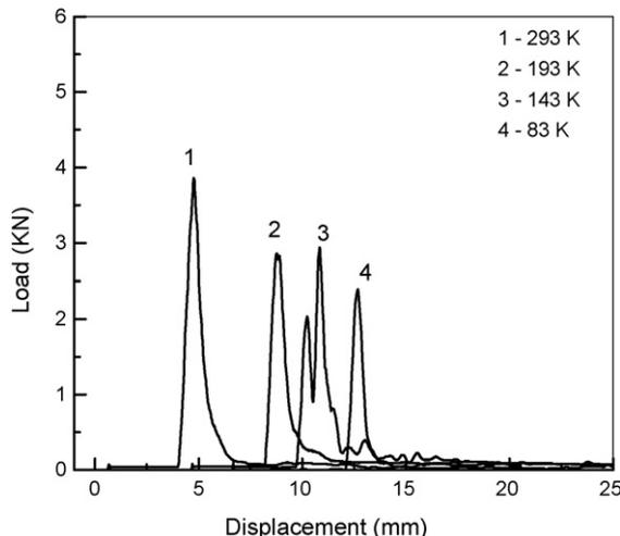
Fig. 2. Load–displacement curves of Ti–2.5Cu at different temperatures.
