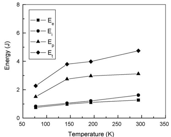
Fig. 3. Crack energies as a function of temperature.  $E_e$  is the elastic energy,  $E_i$  the initiation energy,  $E_p$  the propagation energy and  $E_t$  is the total energy.
